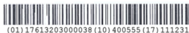
Fig. 4 GS1-128 barcode for health, AIs (17) expiry date, and (10) lot number (Source: General EAN.UCC Specifications, January 2005 - Version 6.0, Section 2.7 - Page 6)
