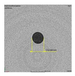
Figure 4. Zoomed-in cross section of the microtube shown in Figure 3 for the determination of inner diameter using the  $\mu$ -CT method. The average inner diameter of the soda glass microtube measured at nine different positions is (0.1269  $\pm$  0.0010) mm.
