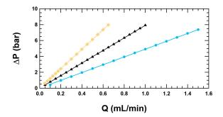
**Figure 6.** Pressure drop as a function of flow rate for the laminar flow of water through the soda glass micro tube (light blue circle), stainless steel microtube (black triangles) and PEEK Beige microtube (beige diamonds).
