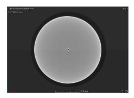
Figure 3. Cross-section of the glass microtube determined by means of  $\mu$ -CT method.
