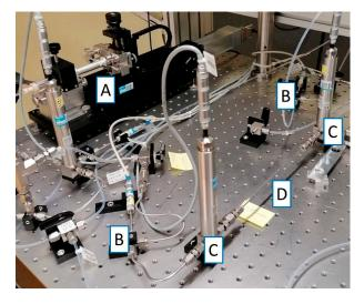
**Figure 2.** The micro pipe viscometer at METAS: (**A**) piston prover, (**B**) temperature sensors, (**C**) pressure sensors and (**D**) the glass microtube with an inner diameter of 0.13 mm and a length of 200 mm.
