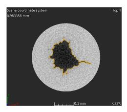
**Figure 5.** Cross-section of the stainless steel microtube determined by means of the  $\mu$ -CT method. Due to the noncircular shape of the cross sections, the volumes were determined to calculate an equivalent inner diameter as (0.144  $\pm$  0.010) mm.
