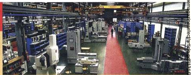
Big and accurate: SIP manufactures the twin-spindle SIP 5000 (left), which can machine a 4-ton workpiece with 3 \mu\text{m} accuracy.
