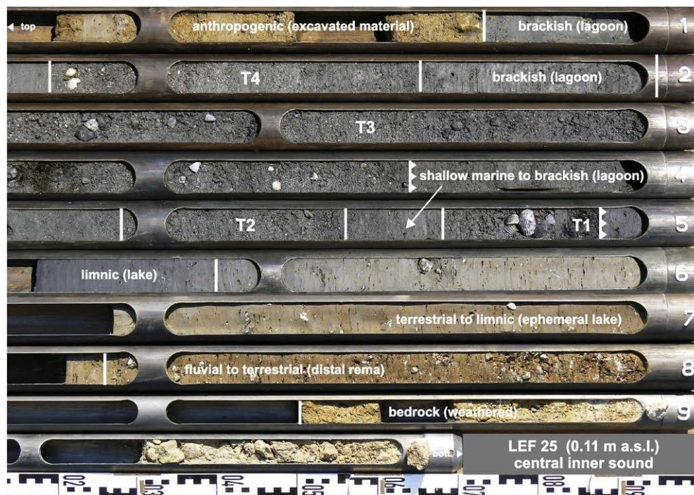
Fig. 4. Facies profile of vibracore LEF 25 from the central inner sound showing a sequence of autochthonous lagoonal mud deposits intersected by four coarse grained tsunami layers out of sandy to gravelly material of marine origin (T1 to T4). The bases of T1 and T2 are characterized by erosional unconformities. Photo taken by M. May, 2006.
