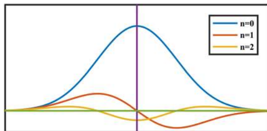
Figure 1. The different order derivatives of absorbance line shape. The 2f signal shape is drawn as a yellow line.
