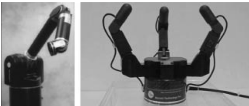
Figure 2. Magilla's (a) arm and (b) hand. Photographs courtesy of Barrett Technologies.
