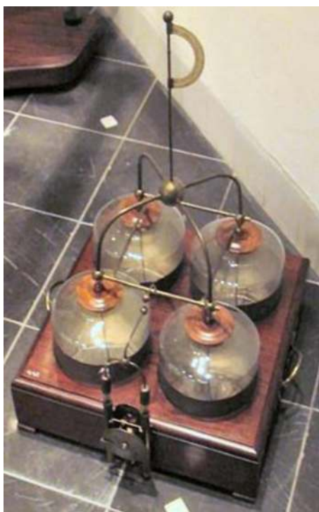
FIG. 17. A “battery” consisting of four water-filled Leyden jars. Photograph attributed to Leidse Flessen Museum Boerhave, Leiden, the Netherlands, licensed under the Creative Commons Attribution-Share Alike 3.0 Unported.
