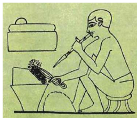
FIG. 12. A photograph of a wall painting found at Thebes in the tomb of the Vizier Rekh-mi-re on the west bank of the Nile River, across from the modern city of Luxor, Egypt, ~800 km south of the Mediterranean Sea. The image, dating from about 1475 BC, depicts a metal worker engaged in brazing at a workshop attached to the nearby Temple of Amun, at Karnak (east bank). He is using a reed tipped with clay for a blowpipe and tongs to hold the parts to be brazed in a charcoal fire in a clay bowl. Adapted from Ref. 40.
