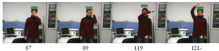
Fig. 6. Part occlusions: occluded by hand (from frame 87 to frame 89), and by arm (from frame 119 to frame 121). The red rectangle shows the position of face obtained by tracking mechanism. The person's identity is obtained by recognition, and showed above face.
