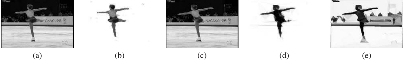
Figure 4. An example of temporal coherence cues. (a) is one frame in the skating sequence and (b) is the figure/ground mask we have obtained. (c) shows the next frame. The two frames (a) and (c) are both represented as triangulations, and we compute a region correspondence/assignment between the two sets of triangles. The correspondence is used to transfer the mask (b) into (d), the spatial “prior” that a triangle in frame (d) supports the object, dark meaning high probability. At the same time, we maintain an appearance model, as brightness histograms of both the object and the background. The appearance prior, or the likelihood ratio of the two histograms, is visualized in (e). In this example, when no color information is available, the appearance prior (e) fires on many parts of the background, while the spatial prior (d) is more focused on the figure.
