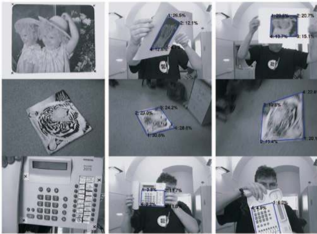
Fig. 14. Ground-truth sequences. The left column shows images used for training. The middle and right columns demonstrate some successfully tracked frames with strong motion blur from the testing sequences. A blue rectangle delineates the object. Percentage values in corners are current corner speeds related to the current size of the object upper edge.
