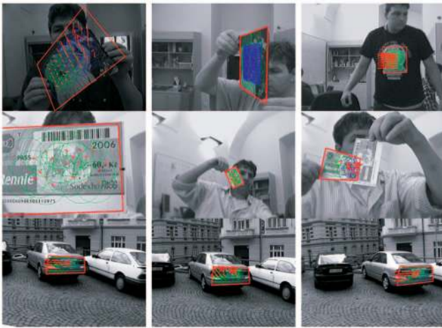
Fig. 11. Robustness to partial occlusions and fast motion: Green/blue circles outline inliers/outliers and red arrows show local motion estimated by SLLiPs. Support set is outlined by blue points.
