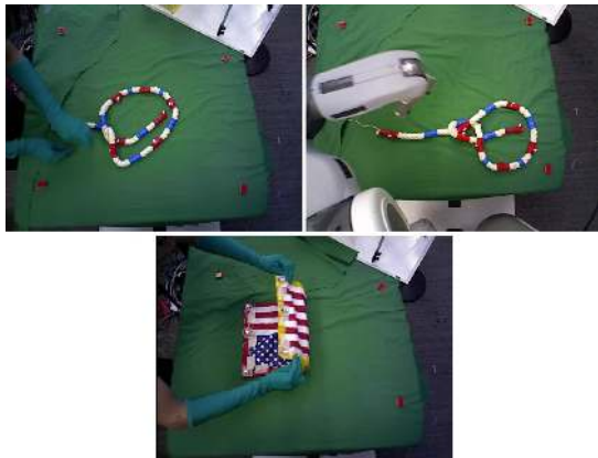
Fig. 6: Manipulation experiments during ground truth data collection with active marker system: human ties a knot (upper left), robot ties a knot (upper right), human folds a towel multiple times (bottom).
