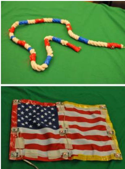
Fig. 5: Ground truth markers on the objects to be tracked.
