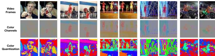
Fig. 3. Temporal Coherence of Color: We visualize frames one second apart from the Kinetics training set [1]. The first row shows the original frames, and the second row shows the ab color channels from Lab space. The third row quantizes the color space into discrete bins and perturbs the colors to make the effect more pronounced. Unlabeled video from the web often has temporally coherent color, which provides excellent, large-scale training data for learning visual trackers. The last column shows an exception where a green light is turned on. Figure best viewed in color.
