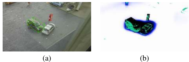
Fig. 2. Simultaneously detecting people and cars. (a) A person and a car is detected, as indicated by the red and green wireframes. (b) The same boxes are projected and filled as black boxes to create a synthetic image that approximates as closely as possible the background subtraction results, shown in green. Note that the white car is the same as the one that appears in Fig. 1 in our introduction section of the main paper. It remains undetected because the background subtraction algorithm fails to extract it.
