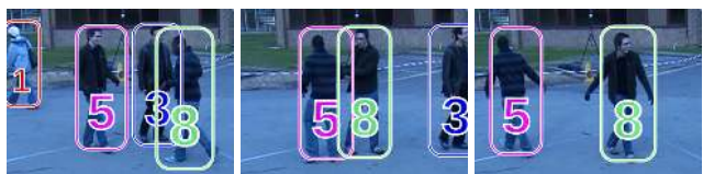
Figure 7. Failure case: Despite the global appearance model, individuals 5 and 8 are switched because of similarly colored clothes.
