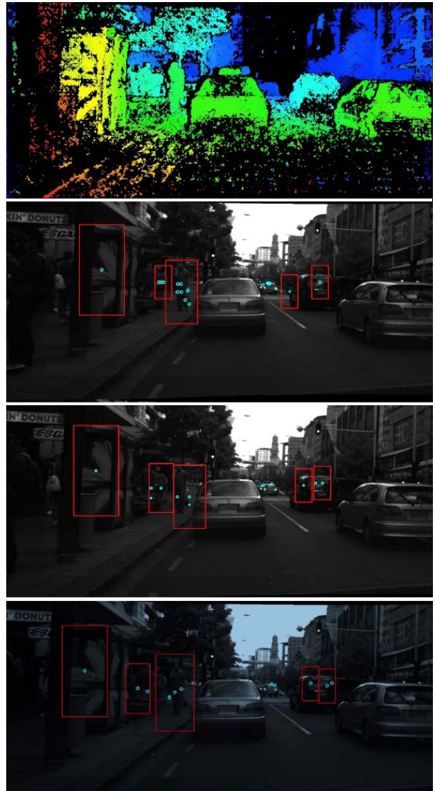
Fig. 1. The depth map on top uses a colour code for calculated distances; depth values are only shown at pixels where the mode filter accepts the given value. The lower images show detected (coloured) object boxes.
