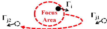
Figure 7. Focus Area. Kinematic constraints are less reliable across larger time windows. Because player motions are globally correlated, the affinity of two mid-level trajectories over large windows should agree with the overall movement trend of the focus area.
