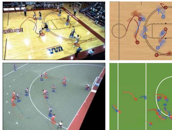
Figure 1. Motion Models. A player’s future motion is contingent on the current game situation. The global distribution of players often indicates which team is attacking, and local distributions denote when opposing players are closely following each other. We use contextual information such as this to create a more accurate motion affinity model for tracking players. The overhead views of basketball and field hockey show the input detections and corresponding ground truth annotations. Player trajectories are strongly correlated with both nearby and distant players.
