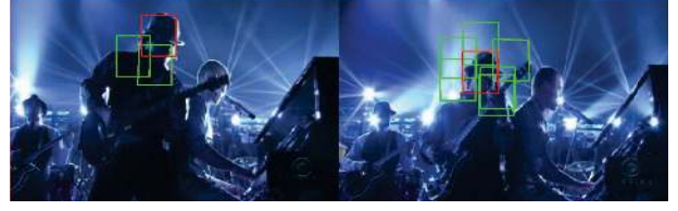
Figure 3. Examples of detected outlier tasks. The green bounding boxes denote the outlier particles and the red bounding box denotes the tracked target. The outliers are detected out of 400 sampled particles. There are two outliers in the left frame and six outliers in the right frame.
