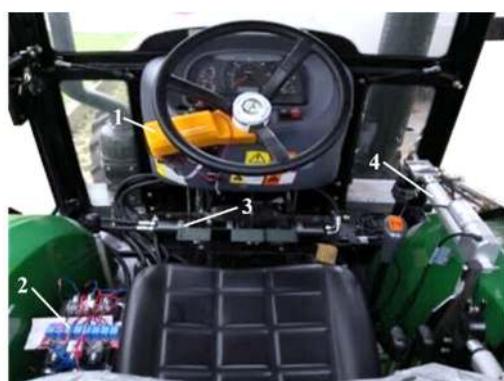
FIGURE 3. The overall arrangement of the driving robot. Among them, 1 is the steering manipulator, 2 is the hydraulic drive, 3 is the pedal control mechanical leg, including a break-leg, a clutch-leg, and a throttle-leg, 4 is the shift manipulator.
