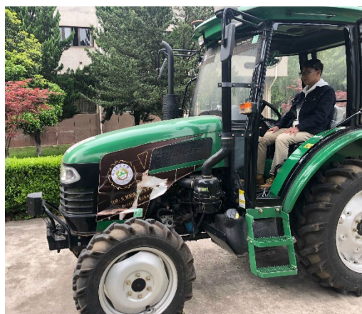
FIGURE 2. The second-generation human-machine cooperative tractor driving robot was developed by our lab which structure is showed in Figure 3. The subjects sat in the tractor and controlled the tractor-driving robot based on EEG signal for straight going, brake, left turn, and right turn.
