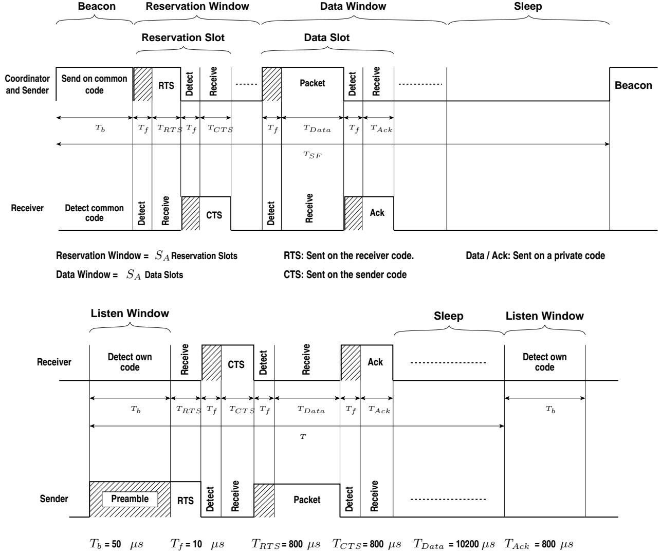
Fig. 2. Sleeping protocols: the Slotted sleeping protocol is depicted on the top. We consider a transmitter and a receiver (and assume this example, that a transmitter is also a coordinator). The protocol defines a superframe. A superframe begins with a beacon sent by a coordinator. It is followed by a reservation window. If a transmitter wants to transmit, it sends a RTS in a reservation slot on the TH code of the receiver (hence concurrent reservations for different receivers are possible). The receiver replies with a CTS if it accepts the reservation. If a reservation is successful, the actual data transmission occurs in the corresponding data slot, and is followed by an ACK. In the beginning of a superframe, nodes need a long beacon to achieve a coarse level synchronization. Afterward, there is only a short preamble before every packet. In the unslotted sleeping protocol (bottom), every node has a regular interval of duration T , called listening schedule. Reservations are done during the listen window at the beginning of the interval, and if successful, are followed by packet transmission. Since a pause between two reservation periods can be long, we need a long preamble at the beginning. One packet at most can be received during T .
