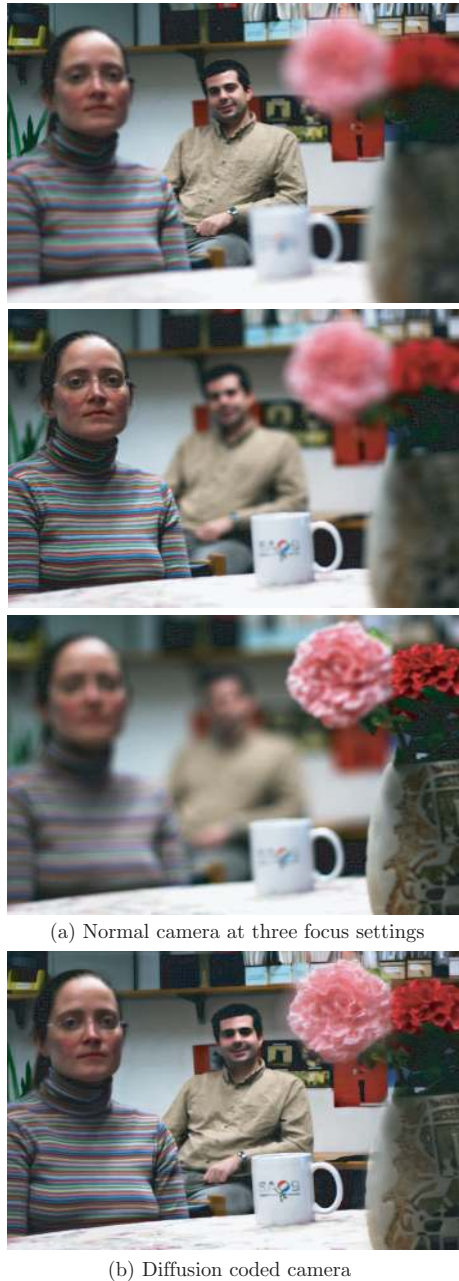
Figure 2.13: Extending DOF with diffusion coding. All images were taken with a 16ms exposure time. (a) The top, middle, and bottom images were captured using a 50mm f/1.8 Canon lens focused on the background, middle, and foreground, respectively. The depth of field is too narrow for all objects to be in focus simultaneously. (b) The diffuser from Section 2.6 is inserted into the lens aperture and deblurring is applied to recover the EDOF image in (b). Diffusion coding results in a roughly 10\times increase in DOF.
