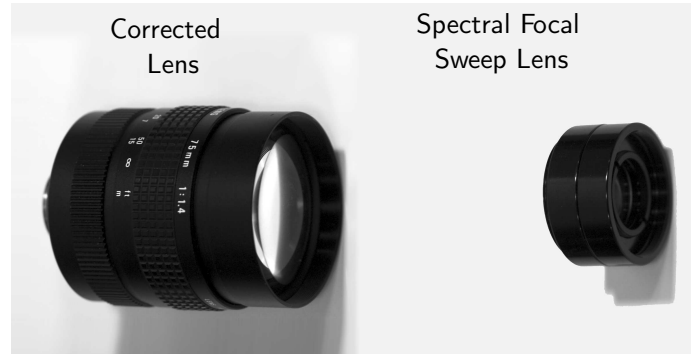
Figure 3.2: A comparison showing the relative sizes and complexities of a Cosmocar 75mm F/1.4 lens (left) and our F/4 SFS doublet lens (right). Our lens is significantly lighter and more compact. The corrected lens is stopped down to F/4 in all experiments.
