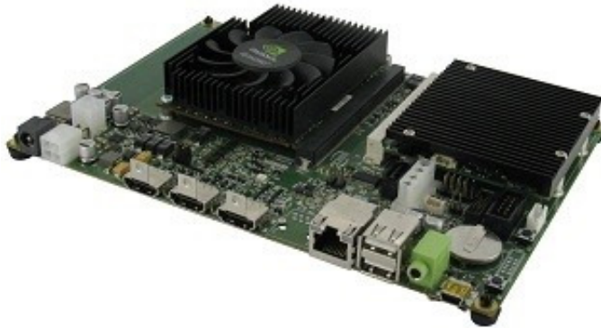
Figure 2: SECO board, which includes a quad-core ARM processor and a Quadro GPU.
