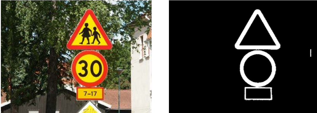
Figure 6.6: Sensitivity to connected signs.
