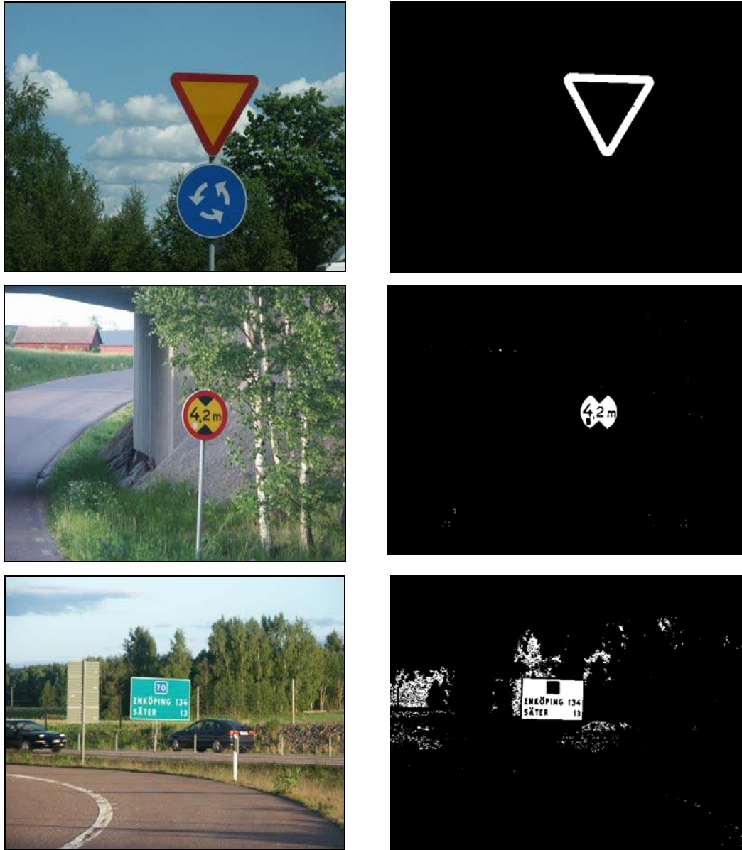
Figure 5.9: Results of applying the modified version of de la Escalera algorithm.
