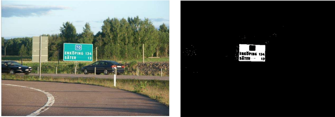
Figure 5.14: Segmentation results from fuzzy colour segmentation algorithm.
