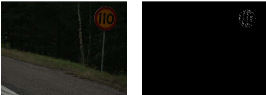
Figure 6.4: Yellow Instability because of low illumination.
