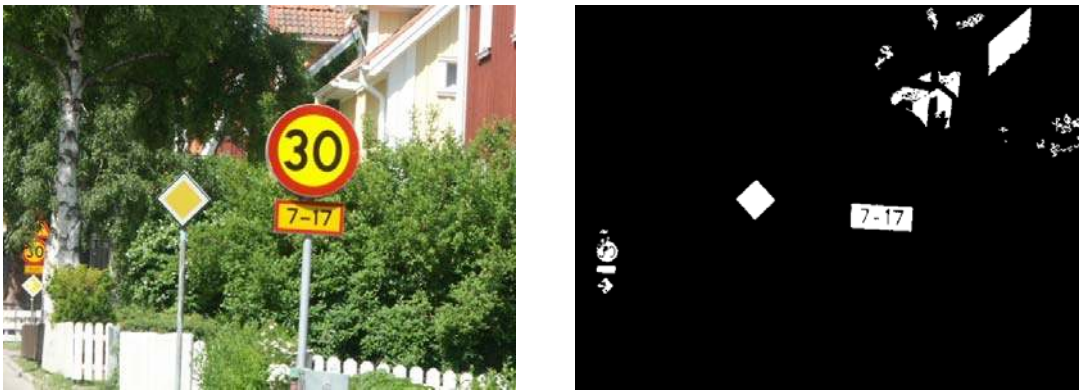
Figure 6.3: Instability of segmentation with yellow.
