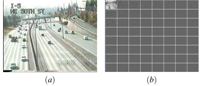
Fig. 2. (a) An I frame from 352 \times 240 input video (b) magnitude of the 8 \times 8 DCT block matrix. Upper left is the DC values.
