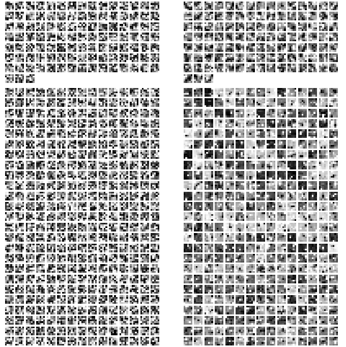
Fig. 4. 5x5 convolution filters for the first stage (top) and second stage (bottom). Left: Random-features ConvNet reaching 97.33% accuracy (see Table III), with 108 and 16000 filters for stages 1 and 2 respectively. Right: Fully trained ConvNet reaching 99.17% accuracy, with 108 and 8640 filters for stages 1 and 2.
