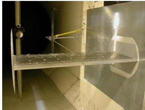
Figure 2 - CCA wind tunnel model mounted in the TDT (looking downstream).
