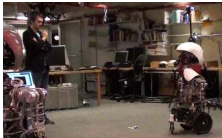
Fig. 1. A training session with the MDS robot Nexi. The artifact used for trainer interaction can be seen on the floor immediately behind Nexi, and the trainer holds a presentation remote by which reward is delivered.
