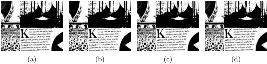
Fig. 2. Salt and pepper noise affecting single pixels occurring with a probability of 0.01; (a) unfiltered, (b) 1 iteration of median, (c) CA, (d) B-rule CA
