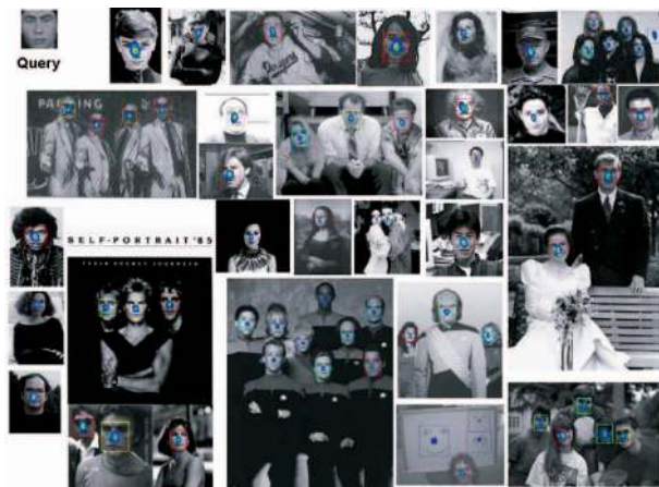
Fig. 17. Detection results on the MIT-CMU multiscale test set [54]. \alpha was set to 0.99. Hand-drawn faces on the white board were also detected using a real face query image.
