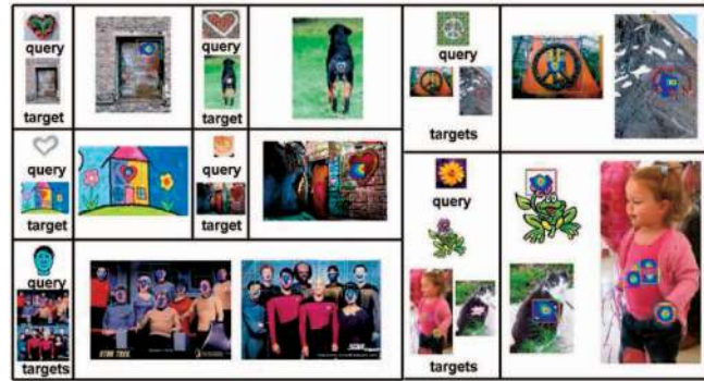
Fig. 23. Query: Hearts, hand-drawn face, peace symbol, and flower. Some targets and examples of correction detections/localizations in Shechtman and Irani's object test set [7] are shown. Some false positives appeared in a girl's T-shirt and candle. \alpha was set to 0.98.
