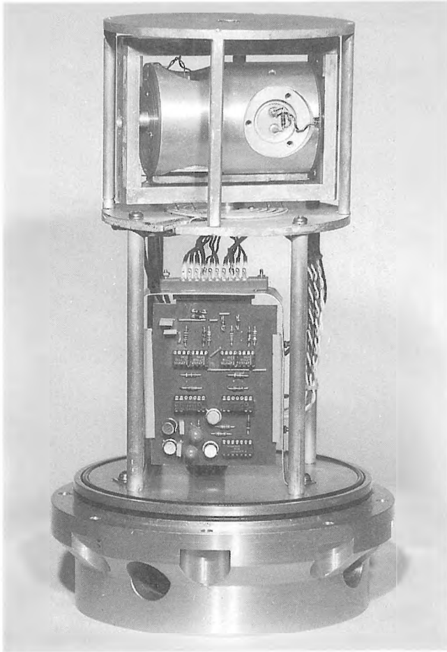
Figure 1 The geophones mounted in gimbals on the OBS endcap. Note the slip rings and the preamps.
