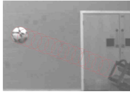
Fig. 3. Data from camera 1 for a launch with no spin. The centers of the circles denote the ball's center of mass in 0.005 s intervals. The ball was launched with speed of v_0 \approx 18 m/s at an angle of \theta_0 \approx 22^\circ from the horizontal.
