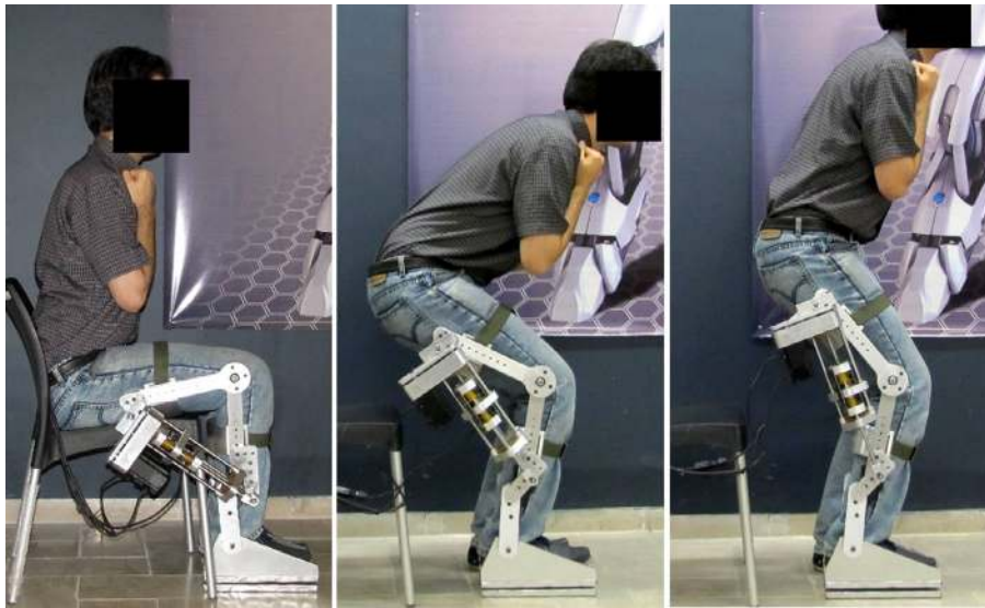
Figure 13. Snapshots from the sit-to-stand movement trials with the assistance of FUM-KneeExo.
