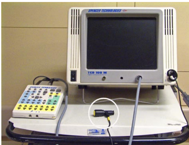
FIGURE 2 M-mode transcranial Doppler machine. Transcranial Doppler probe is shown in the white circle. (Property of Trauma Neuro Critical Care Unit, St. Michael's Hospital, Toronto).
