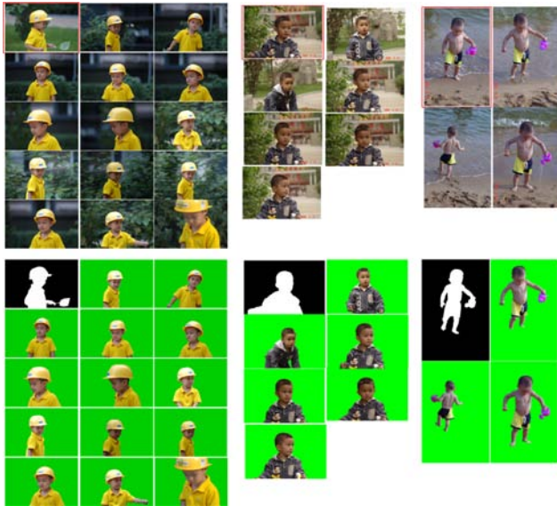
Figure 7. Object cutout for group of images. The images are first clustered into 3 groups. Then in each group one image is selected as an example (marked by the red rectangle). We manually cut out the object from the example image, using the tool [4]. The objects in the other images are automatically cut out as shown.
