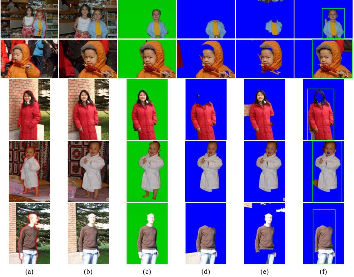
Figure 4. Comparison with state-of-the-art algorithms. (a) is the example image with manually labeled object boundaries represented by red curves, and is used to cut out (b). Our algorithm gets the final result (c). (d), (e) and (f) are the results with S-Induct [13], Co-Seg [12] and GrabCut [11], respectively. Green rectangles in Column (f) indicate the interaction by the user used in GrabCut [11].
