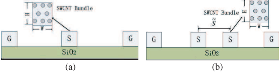
Figure 2. Cross-sectional views of two on-chip CNT bundle interconnects: (a) Ground(G)-signal(S)-Ground(G); and (b) G-S-S-G.
