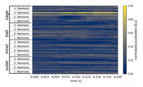
**Figure 5.** An exemplary intermediate domain image for bearing data with four harmonics for each of the four fault frequencies.
