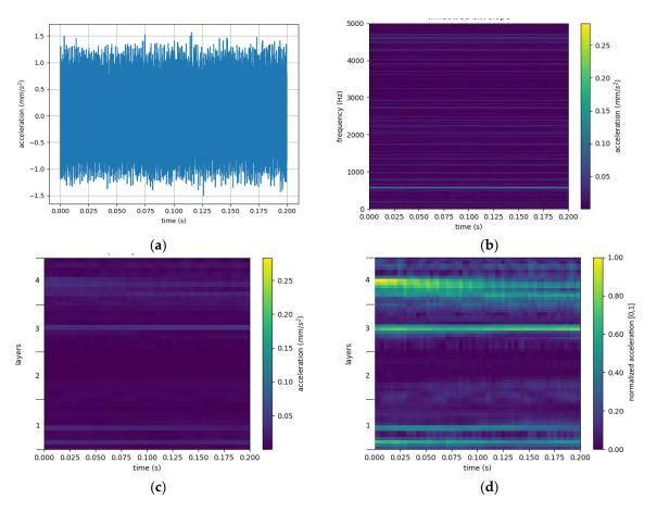
**Figure 4.** The steps of the intermediate domain creation: (**a**) raw sensor data; (**b**) windowed envelope; (**c**) the frequency selective filter; (**d**) final intermedia domain image (after normalization and scaling). The layers in (**c**,**d**) correspond to the following fault areas of a bearing: 1: outer; 2: inner; 3: ball; 4: cage.
