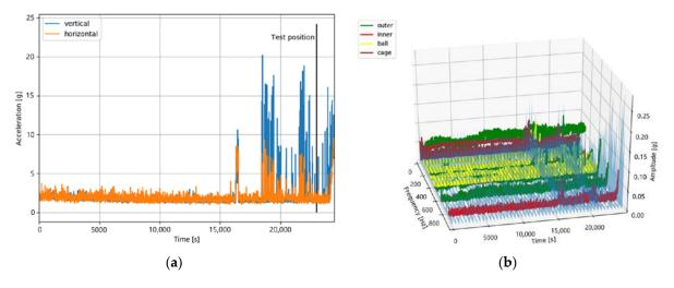
**Figure 14.** The sensor values of bearing dataset 1\_6 in the time domain (**a**) and in the time–frequency domain (**b**). Both plots show no increased measured values at the test position after 23,020 s.
