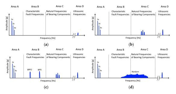
**Figure 11.** The four bearing degradation stages: (**a**) stage 1, contains the rotation frequencies and ultrasonic frequencies; (**b**) stage 2, the natural frequencies of the bearing become visible; (**c**) stage 3, the characteristic fault frequencies appear; (**d**) stage 4, the frequencies in area B and area C are replaced with random noise.
