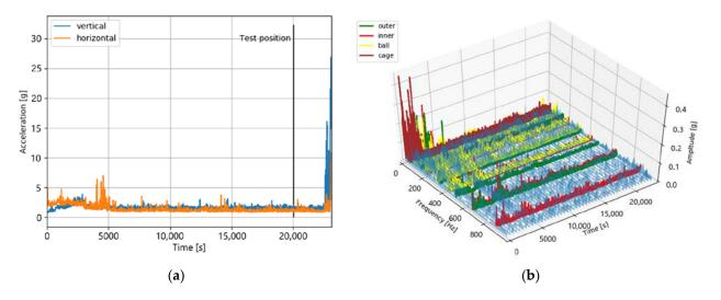
**Figure 13.** The sensor values of bearing dataset 2\_5 in the time domain (**a**) and the time–frequency domain (**b**). Both plots do not indicate a degradation at the test position.
