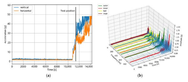
**Figure 12.** The sensor values of bearing dataset 1\_4 in the time domain (**a**) and in the time–frequency domain (**b**). Both figures show increased amplitudes at the test position.
