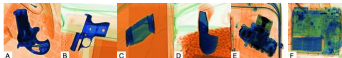
Fig. 3: Bag of visual words approach for multi-class problem. Type of baggage objects and the number of samples in our dataset is as follows: (A) Guns, (B) Gun Components, (C) Knives, (D) Ceramic Knives, (E) Cameras, (F) Laptops
