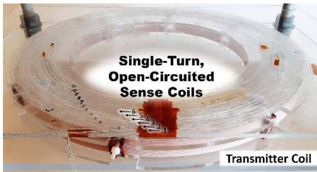
Fig. 24. Sense coils are in the flat plane above the Tx coil.
