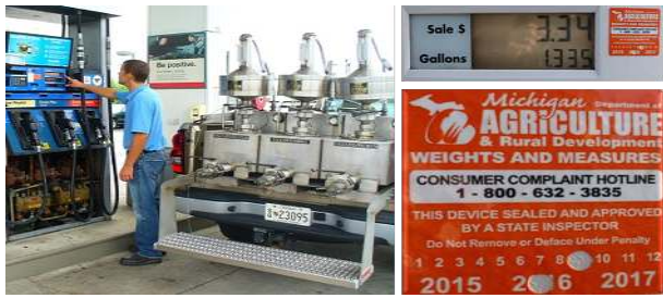
Fig. 3. US Weights and Measure Program qualifies secured gas pump metering (left) with a seal (right). [Photo (left): Weights and Measures, Maryland Department of Agriculture]
