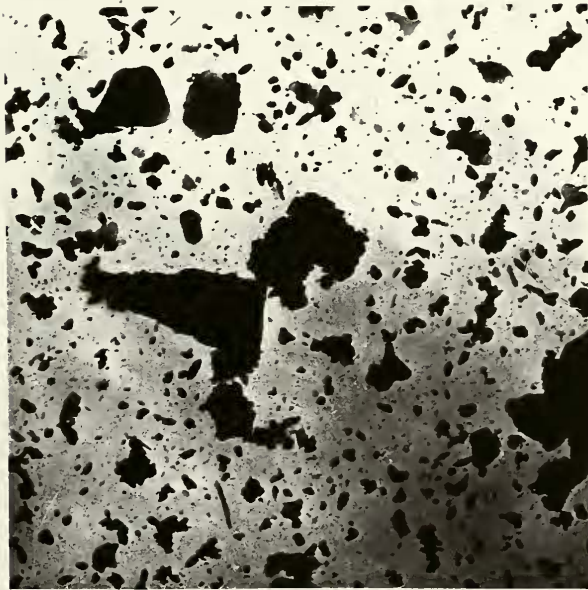
Plate 2. Electron Micrographs of \text{Ca}(\text{OH})_2 -Silicate Reaction Products at 45^\circ\text{C} . (C) Montmorillonite. (D) Mica
