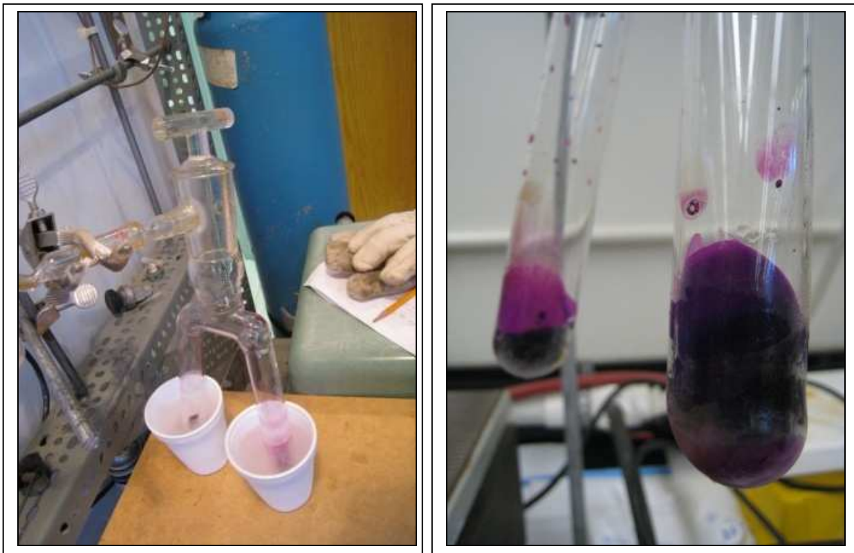
Figure S1: (Left) The Rittenburg tube containing \text{MnO}_4^- solution was frozen in liquid nitrogen while all gases were being vacuumed. (Right) thawed RDX- \text{MnO}_4^- solution after mixing.
