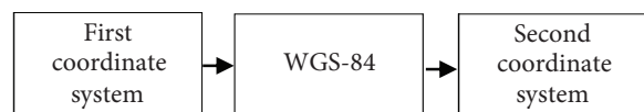
Figure 1. Standard software scheme for the transformation from one coordinate system to another
