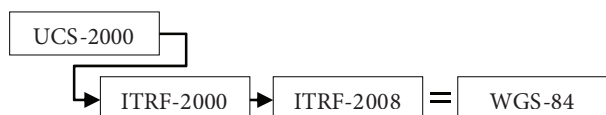
Figure 2. The scheme of coordinate transformation from UCS-2000 to the new realization of WGS-84
