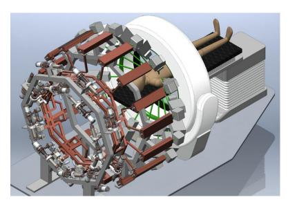
**Figure 15.** Conceptual diagram of the PHASER architecture with 16 linacs arrayed around the patient for highly conformal FLASH photon therapy. Reproduced with permission from Ref. [141].
