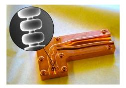
Figure 18. SLAC mm-wave linac prototype for high-power testing.
