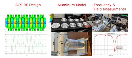
**Figure 5.** Design, cold model, and measurements of the annular-coupled structure (ACS) developed by Argonne in collaboration with RadiaBeam.
