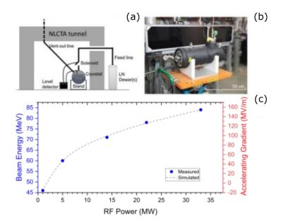
**Figure 16.** (a) Schematic of cryogenic test setup at XTA using liquid nitrogen. (b) Photo of linac and cryostat assembly prior to installation at XTA. (c) Measurements of accelerating gradient as a function of RF power.
