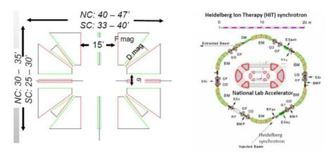
**Figure 7.** Outer dimensions for a variable energy 330 MeV/nucleon therapeutic ring (**left**) and a dual ring system of 430 MeV/nucleon (**right**) compared with the Heidelberg ion therapy facility. On the right, the FLASH-capable, CW, and variable-energy 430-MeV/nucleon ion accelerator nested system is compared to equivalent-energy, low-duty-cycle Heidelberg ion therapy synchrotron. Inner ring racetrack is 250 MeV/nucleon and can provide independent beam delivery.
