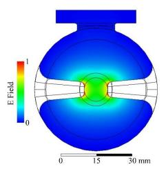
**Figure 19.** Electric field profile of the TE11-like mode shown in a cross-section of the deflector cell, with beam axis oriented into the page. The opposing posts (profiles shown in white) produce an RF dipole. Power is coupled in through the port at the top of the model simulated in ANSYS-HFSS.
