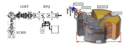
**Figure 9.** HIMAC, Japan ion source, and RFQ (**left**), which serve as the concept for the upstream pre-acceleration system for the injector accelerator (**right**). A CAD model of the full conceptual design of the 20 MeV/u injector system (scalable to 70–100 MeV/nucleon) is shown on the right. From left to right, the ECR ion source, focusing solenoid, RFQ, beam focusing quadrupoles, and the cyclotron shown with a transparent outer shielding for clarity.
