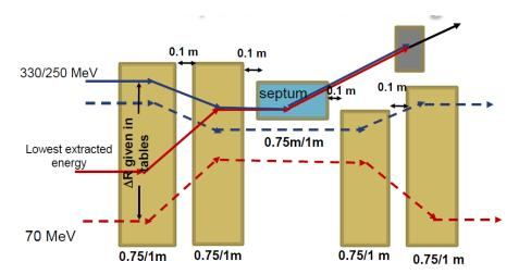
**Figure 8.** Layout of the ramped, bipolar magnet extraction system that selects the orbit and energy for extraction through a septum. Inner, lower-energy orbits are returned to their respective closed orbits for continued acceleration. Reproduced from Ref. [50].
