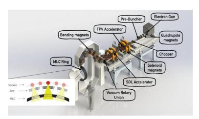
**Figure 13.** Rendering of the ROAD FLASH-RT system. A segment of the decoupled MLC ring is shown in the figure inset with three MLC modules. The linac is triggered to produce the beam when the target is aligned with the MLC to produce a VMAT-like treatment.
