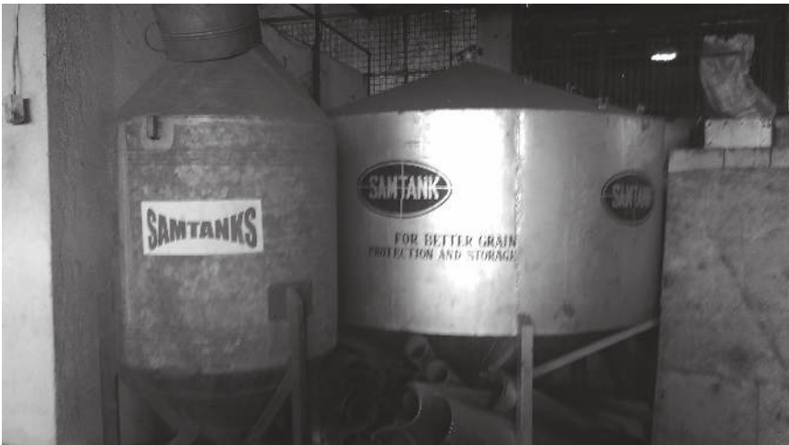
Figure 13.1 Metal silo bins from local production in Tanzania; hermetic seal feasible
