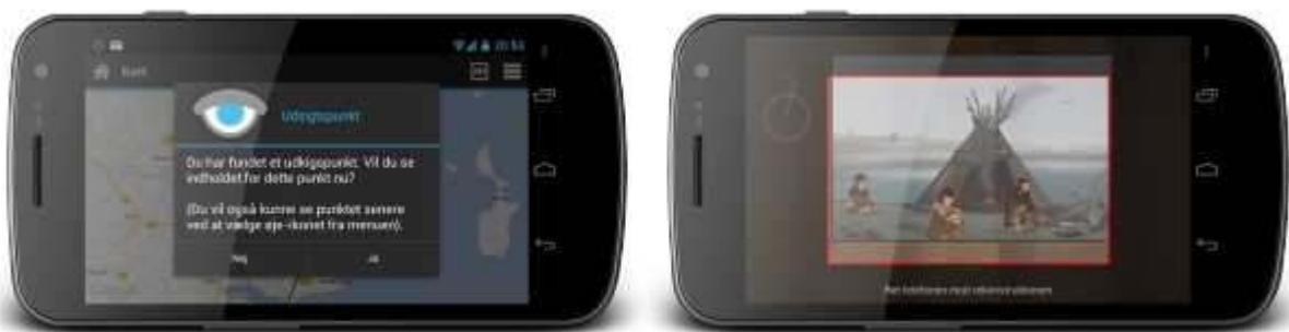
Figure 8: Left: A vista point is found, and if the user chooses to see the content, she will be instructed to hold up her phone and search for the reconstruction (as seen in the picture to the right).
