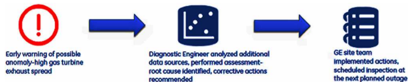
Fig. 3 GE big data diagnostics process for the LNG liquefaction industry segment
