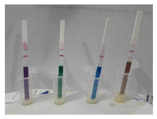
**Figure 11.** Example of test result carried out with farmers. Two lines indicate positive for GMO presence. Photo credit: Semi-arid Agrobiodiversity Management Program and Agrobiodiversity of the Semi-arid Project image bank. Embrapa Semiárido Seed Laboratory, Petrolina, Pernambuco, Brazil, January 2021.
