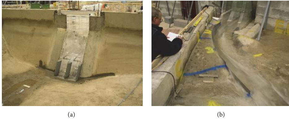
FIGURE 5: Physical hydraulic model of the bottom outlet. (a) Upstream view; (b) downstream view with free outflow.
