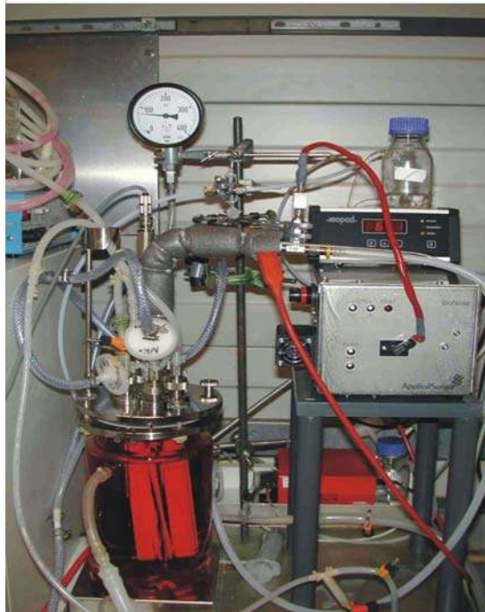
Fig. 2.15.1a: The bioreactor and BioNose set up. (Obtained from EU BioNose Project QLK3-CT-1999-00435).
