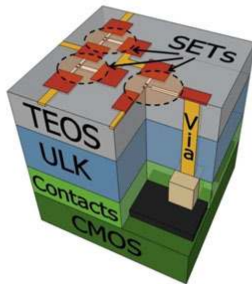
Figure 1: Cross section of the 3D hybrid SET-CMOS integration in the BEOL.
