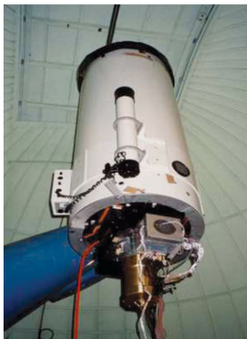
Figure 1. The Boller and Chivens (B&C) telescope with the CCD camera MOA-cam2. The telescope has a 61-cm aperture Richey-Chretien Cassegrain reflector and the camera has three 2048 \times 4096 pixels SITE thinned back-illuminated CCD chips (ST-002A).
