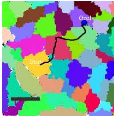
Fig. 6. A simulated environment fully explored. Each region represents the place field of a particular place cell. After a full exploration, the entire environment is covered by the place cell population. The curve is an example of a planned path to reach a goal place (presence of a source).
